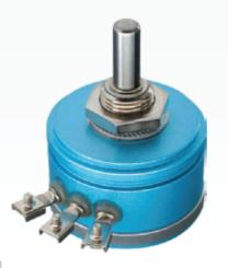
The product line of the low torque resistors stands out due to the extremely low torque of 0,003 Ncm, which enable a very sensitive adjustment. In order to achieve this torque, the contact pressure of the tapper on the winding is kept as low as possible. The rotatable resistors consist of a wound resistance and a slider, which is coupled to the needle shaft of the measuring device by a clutch system. For tapper and winding only noble-metal alloys with high corrosion resistance are used.
